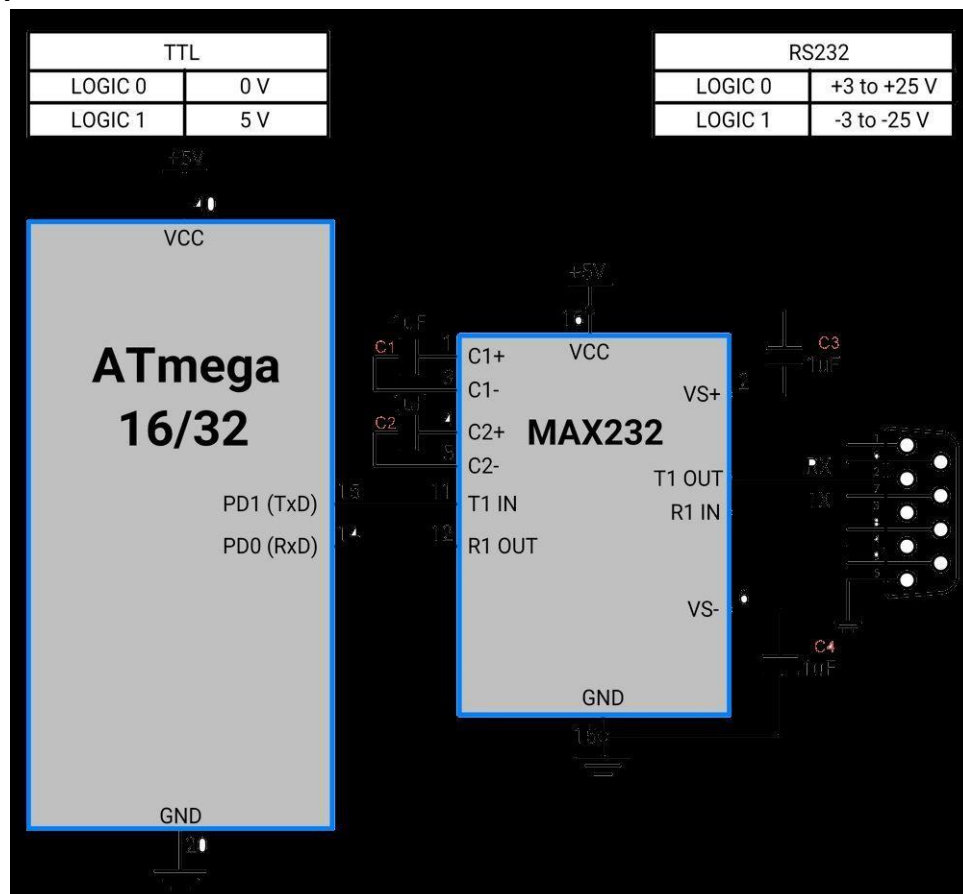
ATmega16/32 Serial Interface Connection Diagram
